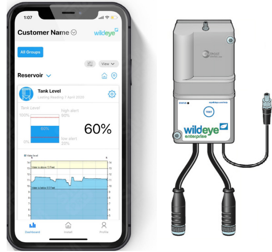
Wildeye 3G/4G IoT logger - rechargeable, 2 plug version with example iPhone app screenshot
